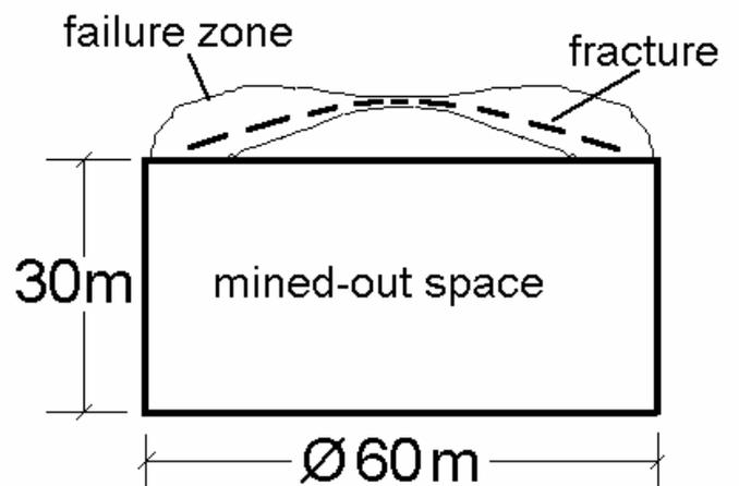
Figure 2. Failure zone above the mined-out space
