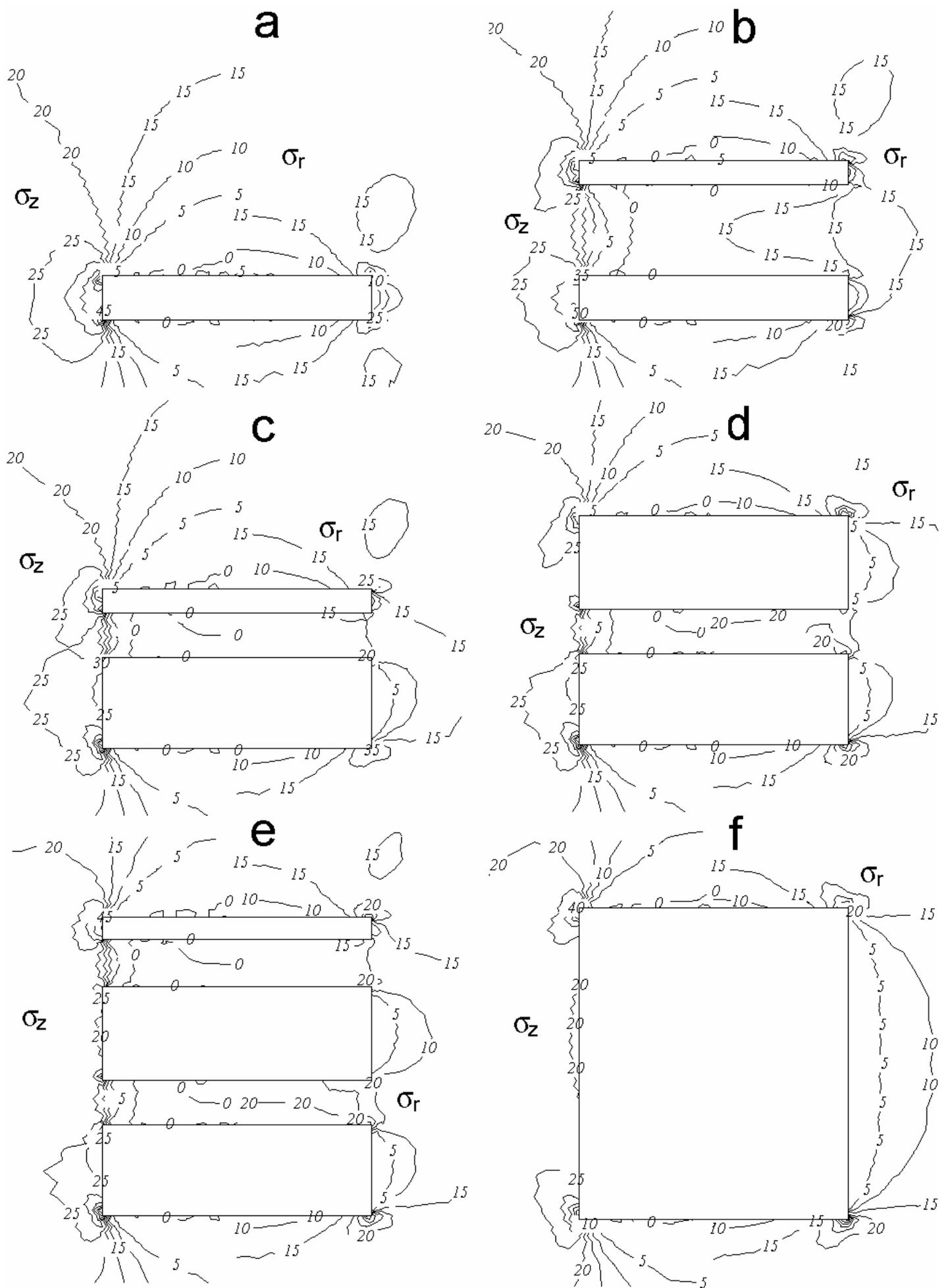
Figure 1. Vertical (left) and horizontal radial (right) components of stresses (MPa) in rock around mined- out spaces at consecutive extraction of ore in experimental industrial block of “International” Mine at the depth of 800 m ( $\lambda=0.8$ ).
