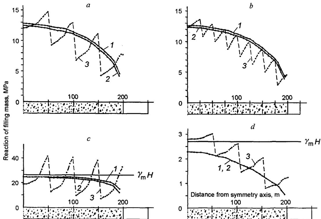
Fig. 1. Reaction of filling mass with successive increase in width of the mined-out space filled with stowing to 400 m, according to calculations in the direct formulation (1) and in terms of the final additional stress (2) and calculations where the sequence in which the artificial mass is created is taken into account (3).
