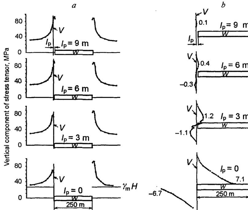
Fig. 4. a) Support pressure in successive approaching operation front to a vertical geological disturbance; the distance from the fracture to the boundary of mined-out space decreases from 9 m (upper graph) to 0 m (lower graph); b) shear of the sides of a vertical geological disturbance (cm) as the mined-out space approaches;  $W$  denotes the mined-out space, and  $V$  denotes the vertical fracture.
