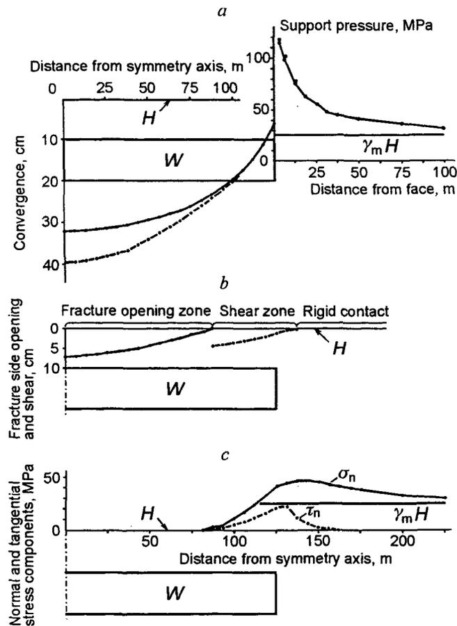
Fig. 5. Convergence of roof and floor of the mined-out space and support pressure without fracture (solid curves) and with (dash-dot curves) a horizontal geological disturbance (a), opening and slip of fracture sides (b), and distribution of the normal and tangential stress components at the fracture surface (c);  $W$  denotes the mined-out space, and  $H$  denotes the horizontal fracture.
