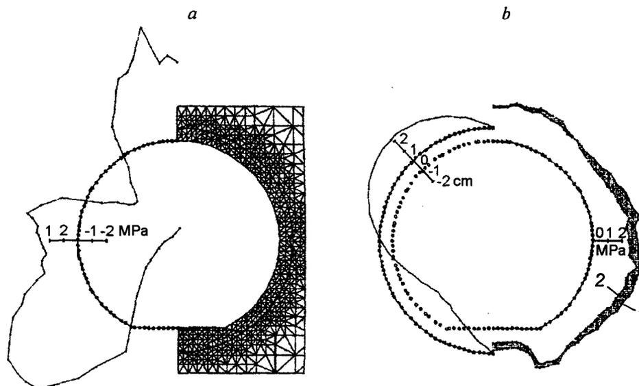
Fig. 2. Discretization of the region into triangular elements close to the tunnel (*a*, on the right), stress distribution at the inner tunnel contour in the direct formulation (*a*, on the left) and in terms of the additional stresses (*b*, on the right), disregarding (solid curve 1) and taking account of (dash-dot curve 2) slippage at the contact of soil massif with tunnel lining, and the distribution of soil massif shear at the contact (*b*, on the left).
