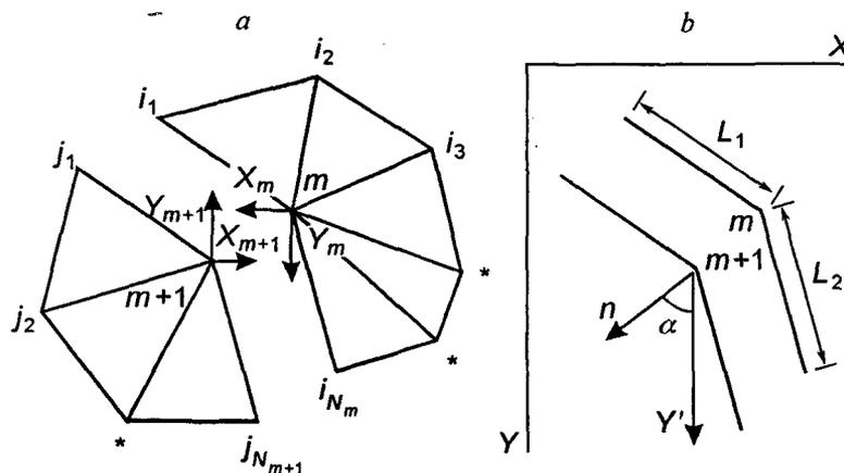
Fig. 3. Double nodes at the contact of soil mass with tunnel lining.
