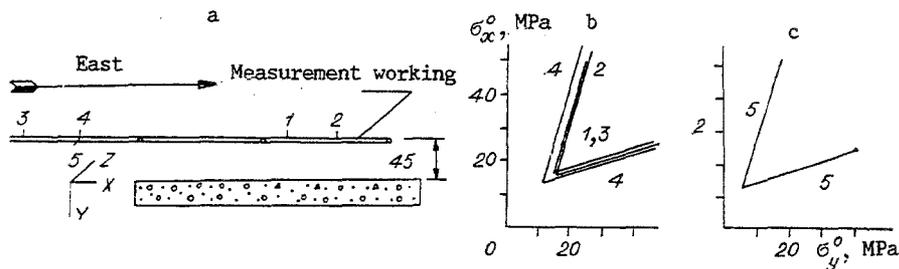
Fig. 7. Vertical cross-section of the central portion of an ore body with location of measurement holes (a) and permissible values of initial stress component (b, c).
