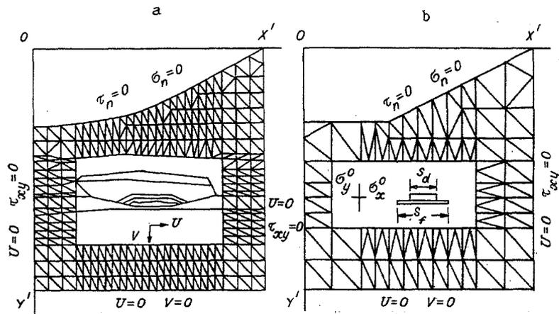
Fig. 4. Detailed (a) and simple (b) grids for solution of two-dimensional problems.
