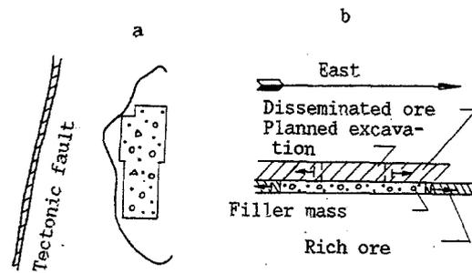
Fig. 1. Plan (a) and transverse cross-section (b) of a mine.
