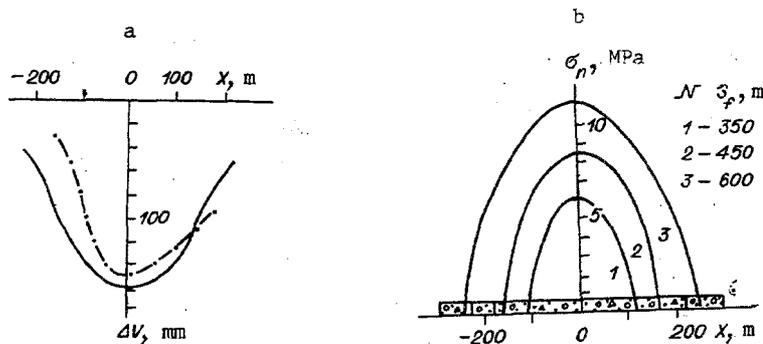
Fig. 6. Vertical displacements of underworked bed (a) and pressure in filling (b).
