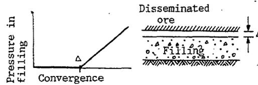
Fig. 5. Support pressure of filler mass as a function of roof and floor convergence.
