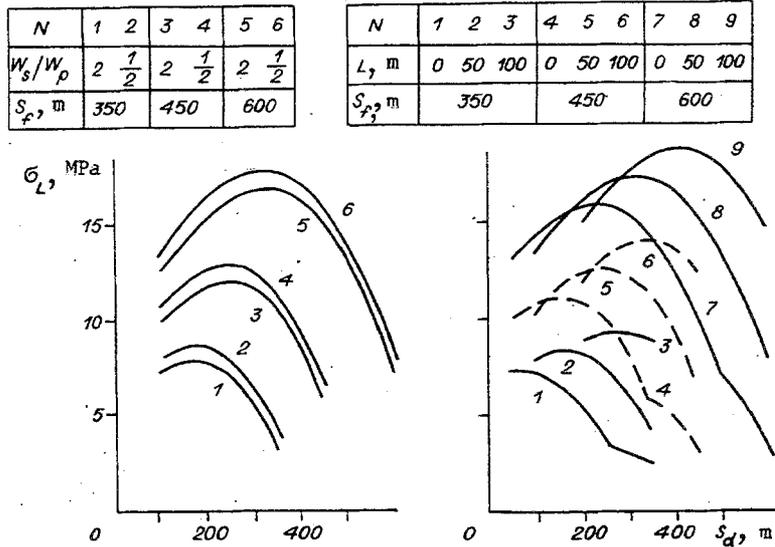
Fig. 9. Vertical stresses at phase of secondary strips as a function of span for various geometric parameter values.
