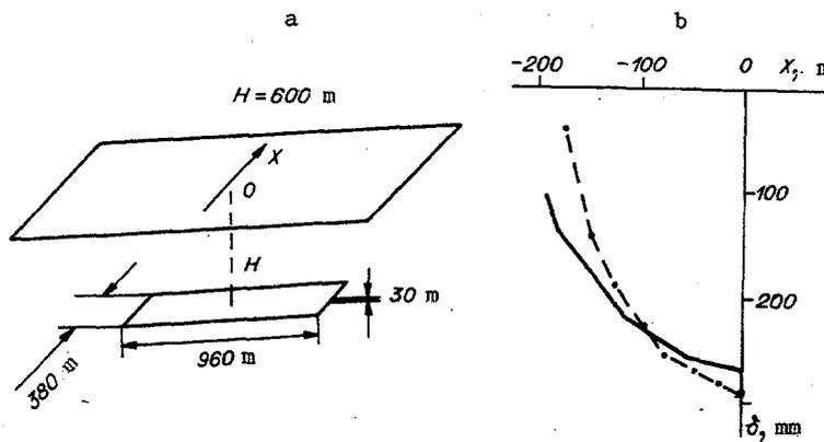
Fig. 3. Calculated region of three-dimensional problem (a) and roof and floor convergence in central cross-section of a cavity (b): solid curve – two-dimensional; dashed curve – three-dimensional.
