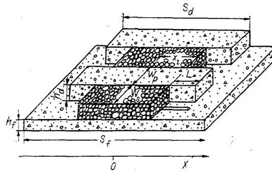
Fig. 2. Excavation layout for disseminated ore by combination method.
