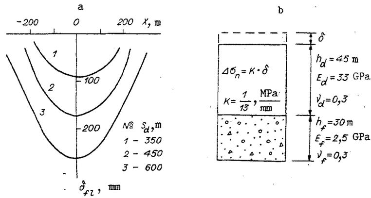
Fig. 8. Additional convergence as a function of span length during complete excavation of disseminated ore (a) and the "ore pillar-underlying filler mass" system (b).
